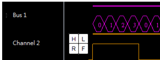
Figure 4-11 Collapsed Bus View
